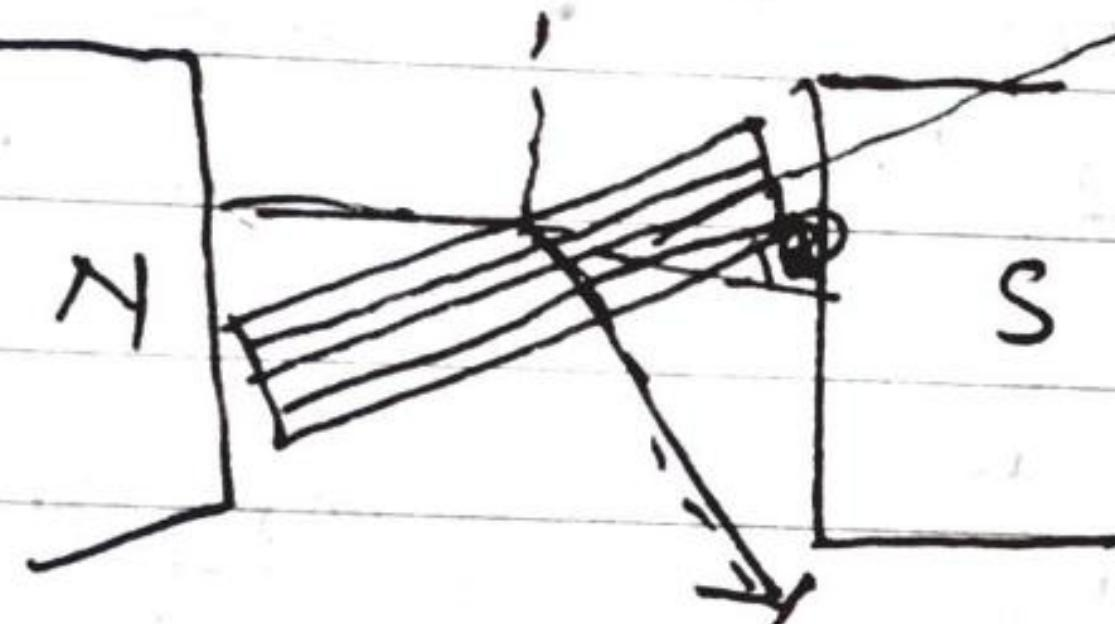
Due to action of this torque the coil is set in rotation about the axis of suspension producing into play in the opposite direction which increases with the increase in the angle of twist and eventually when this torque equals the magnetic torque the coil comes to rest.
